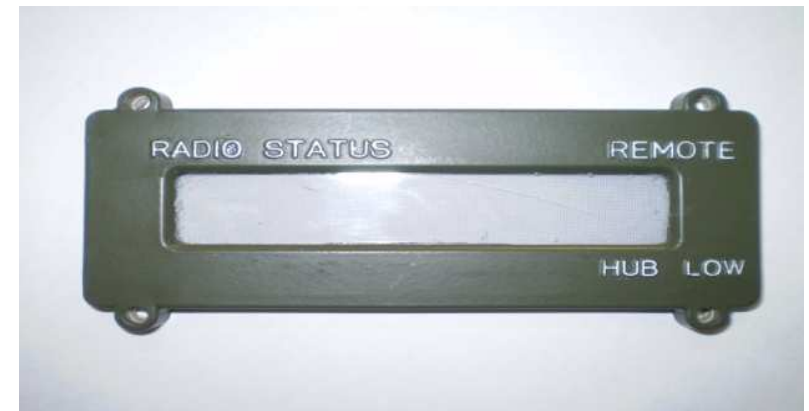
Chemically toughened glass Bonded using Cho Bond between mesh & bezel
