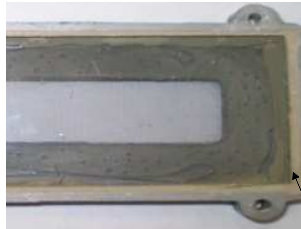
Chemically toughened glass Bonded using Cho Bond between mesh & bezel
